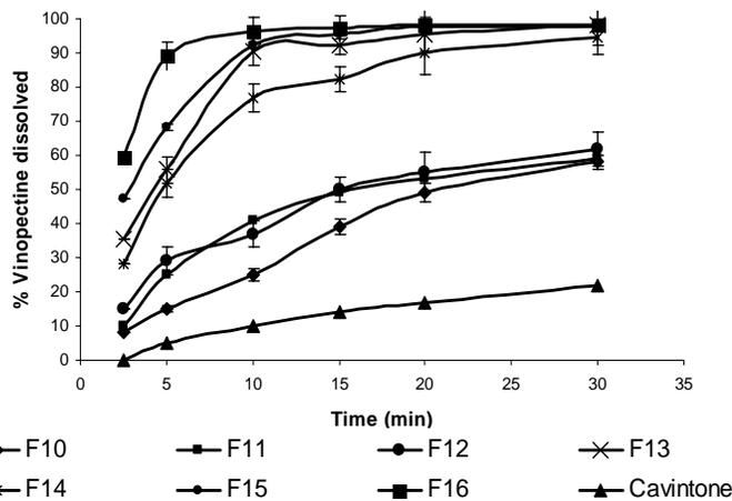
**Figure.6:** In-vitro dissolution profiles of vinpocetine from ODTs prepared by inclusion complex in phosphate buffer pH 6.8 at  $37 \pm 0.5^\circ\text{C}$
