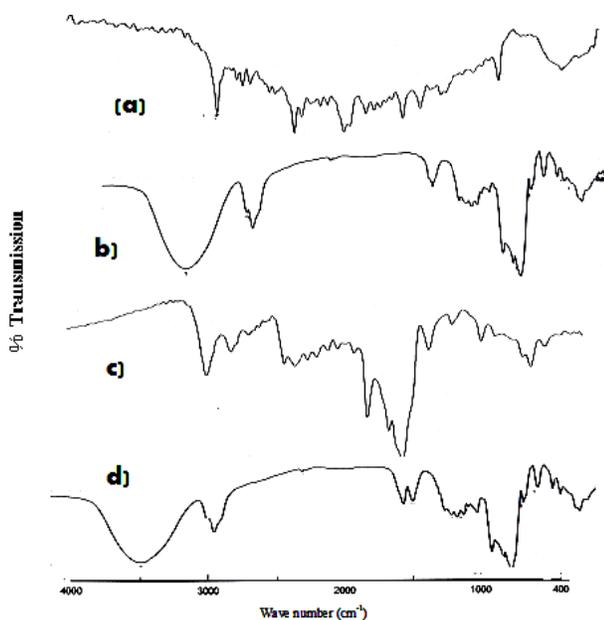
**Figure.4:** FTIR patterns of vinpocetine-2HP  $\beta$ -cyclodextrin solid systems. a) Pure vinpocetine; b) Pure HP- $\beta$ -CD; c) Physical mixture and d) Inclusion complex
