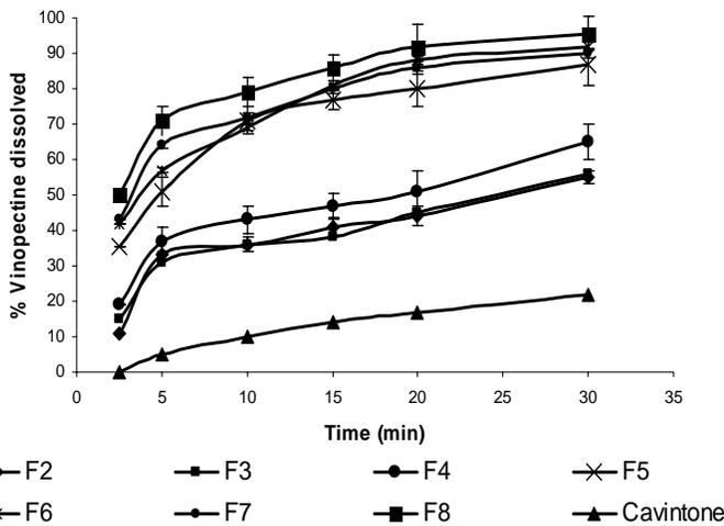
**Figure.5:** In-vitro dissolution profiles of vinpocetine from ODTs prepared by solid dispersion in phosphate buffer pH 6.8 at  $37 \pm 0.5^\circ\text{C}$
